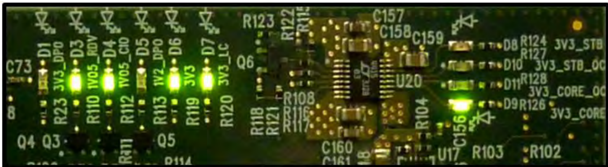
Thunderbolt™ 2 Interface Card LEDs: Functional Mode - without external display device attached
